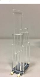
The set of accessories for mouse 35250-003 consists of two special tubes, with a 45x95(h)mm opening, connected by a metal bridge, whose width was minimized to 4cm.
